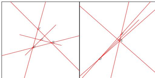
Figure 7: 2D system of 4 points and 5 lines with 10 point-line incidences, 4 angle parameters  $\text{angle}(qp, cp)$ ,  $\text{angle}(cp, rp)$ ,  $\text{angle}(rq, cq)$ ,  $\text{angle}(cq, pq)$  and 1 distance parameter  $d(r, c)$ . Symmetric solution (left) and random, typical witness solution (right).
