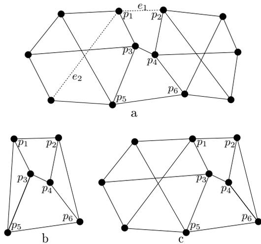
Figure 15: 2D systems where edges represent point-point distances; (a): 3-connected constraint graph made of two  $K_{3,3}$  graphs connected with 3 constraints; (b) and (c): graphs obtained by replacing MRSs identified by Algorithm 8 by their boundary with respectively edges  $e_1$  and  $e_2$  removed.
