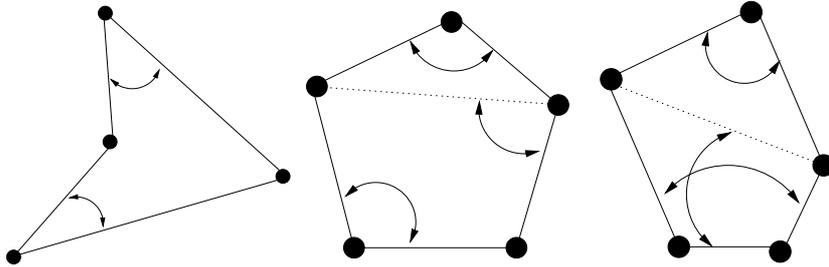
Figure 10: 3D examples (courtesy of Auxkin Ortuzar, Dassault Systèmes) which confuse graph-based methods but are detected over-constrained by our method. No three points are coplanar, plain segments represent distance constraints and arcs represent angle constraints.
