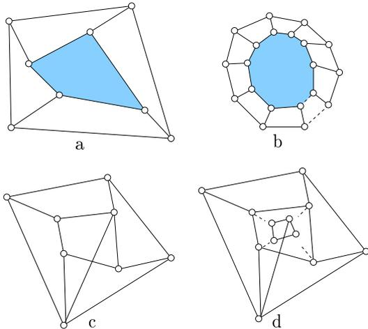
Figure 17: 2D rigid examples for the  $\mathcal{W}$ -decomposition: each vertex is a point and each edge represents a distance constraint. (a):  $\mathcal{W}$ -decomposable 4-connected GCS (the blue subsystem is rigid); (b):  $\mathcal{W}$ -decomposable  $k$ -connected GCS (the blue subsystem is rigid); (c):  $\mathcal{W}$ -indecomposable system; (d): there are  $\mathcal{W}$ -indecomposable systems with an arbitrary number of points.
