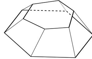
Figure 16: Generalized Stewart platform: both thick hexagons are rigid; the other segments indicate distance constraints.
