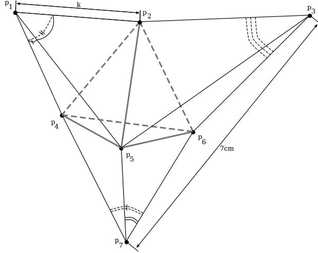
Figure 9: Rigid 3D system decomposable in 4 scalable tetrahedrons and a rigid segment
