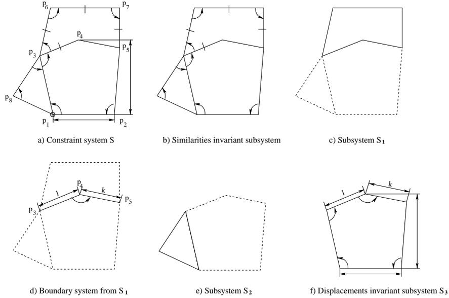
Figure 8: Decomposition of a 2D system into 3 subsystems
